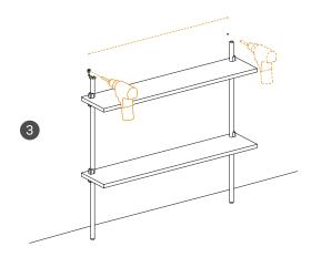
Lean the lower section against the wall, mark and drill the first two mounting holes. These holes must be leveled and 766 mm apart. Use an adequate wall plug suited for your wall type.
