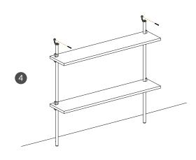
Fix the upper mounting clips with the provided screws.
