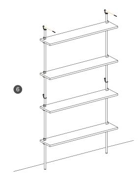
Screw the connector screws as far into the legs as possible. Add the leg extensions by screwing them tight against the lower part of the legs.
