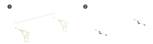
Mark and drill holes for the two upper mounting clips. These holes must be leveled and 766 mm apart. Use an adequate wall plug suited for your wall type.
