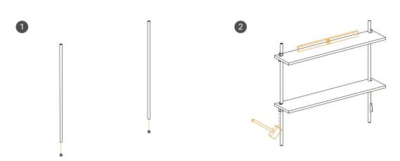
Start by installing two end caps in the bottom of each leg.
